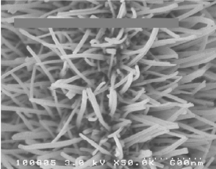
Figure 20.16. As-grown 3M, PR149 whiskers. (Image reproduced courtesy of 3M Corporation.)
