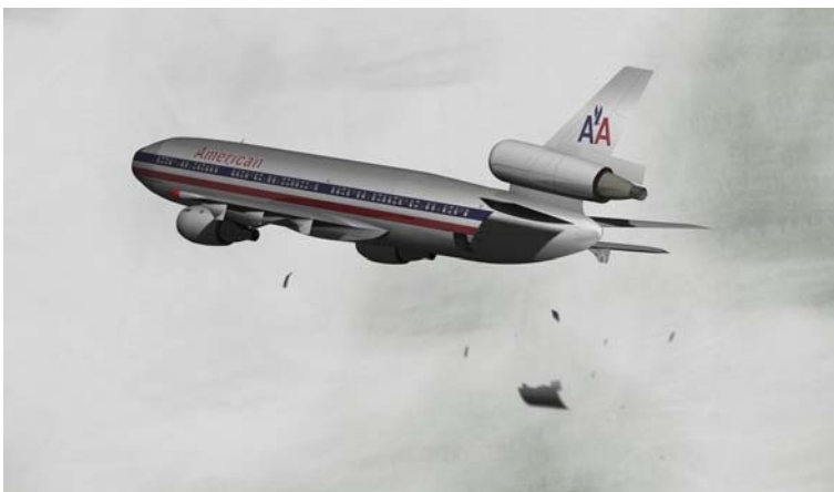
Fig. 3.16 The DC-10, shown in this recreation as it is losing the rear cargo door. [Used with permission, Wikipedia Common, http://commons.wikimedia.org/wiki/File:Aaflight96dc10.png ]
