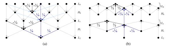
**Figure 3.39** Lifted transform shown as a signal processing diagram: (a) The analysis stage first predicts the odd value from its even neighbors, stores the difference wavelet, and then compensates the coarser even value by adding in a fraction of the wavelet. (b) The synthesis stage simply reverses the flow of computation and the signs of some of the filters and operations. The light blue lines show what happens if we use four taps for the prediction and correction instead of just two.
