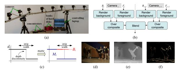
**Figure 13.15** Video view interpolation (Zitnick, Kang, Uyttendaele *et al.* 2004) © 2004 ACM: (a) the capture hardware consists of eight synchronized cameras; (b) the background and foreground images from each camera are rendered and composited before blending; (c) the two-layer representation, before and after boundary matting; (d) background color estimates; (e) background depth estimates; (f) foreground color estimates.
