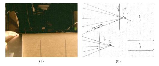
**Figure 6.7** Calibrating a lens by drawing straight lines on cardboard (Debevec, Wenger, Tchou *et al.* 2002) © 2002 ACM: (a) an image taken by the video camera showing a hand holding a metal ruler whose right edge appears vertical in the image; (b) the set of lines drawn on the cardboard converging on the front nodal point (center of projection) of the lens and indicating the horizontal field of view.
