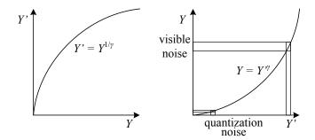
**Figure 2.31** Gamma compression: (a) The relationship between the input signal luminance Y and the transmitted signal Y' is given by  $Y' = Y^{1/\gamma}$ . (b) At the receiver, the signal Y' is exponentiated by the factor  $\gamma$ ,  $\hat{Y} = Y'^{\gamma}$ . Noise introduced during transmission is squashed in the dark regions, which corresponds to the more noise-sensitive region of the visual system.
