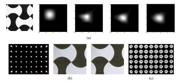
**Figure 10.8** Point spread function estimation using a calibration target (Joshi, Szeliski, and Kriegman 2008) © 2008 IEEE. (a) Sub-pixel PSFs at successively higher resolutions (note the interaction between the square sensing area and the circular lens blur). (b) The radial distortion and chromatic aberration can also be estimated and removed. (c) PSF for a mis-focused (blurred) lens showing some diffraction and vignetting effects in the corners.
