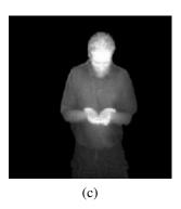
**Figure 12.6** Shape scanning using cast shadows (Bouguet and Perona 1999) © 1999 Springer: (a) camera setup with a point light source (a desk lamp without its reflector), a hand-held stick casting a shadow, and (b) the objects being scanned in front of two planar backgrounds. (c) Real-time depth map using a pulsed illumination system (Iddan and Yahav 2001) © 2001 SPIE.
