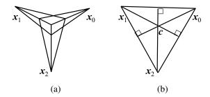
**Figure 6.9** Calibration from vanishing points: (a) any pair of finite vanishing points  $(\hat{x}_i, \hat{x}_j)$  can be used to estimate the focal length; (b) the orthocenter of the vanishing point triangle gives the optical center of the image c.
