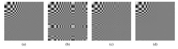
**Figure 2.25** Aliasing of a two-dimensional signal: (a) original full-resolution image; (b) downsampled  $4 \times$  with a 25% fill factor box filter; (c) downsampled  $4 \times$  with a 100% fill factor box filter; (d) downsampled  $4 \times$  with a high-quality 9-tap filter. Notice how the higher frequencies are aliased into visible frequencies with the lower quality filters, while the 9-tap filter completely removes these higher frequencies.
