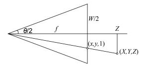
**Figure 2.10** Central projection, showing the relationship between the 3D and 2D coordinates, p and x, as well as the relationship between the focal length f, image width W, and the field of view  $\theta$ .
