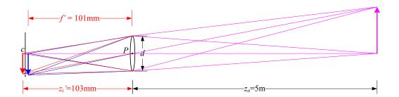
**Figure 2.21** In a lens subject to *chromatic aberration*, light at different wavelengths (e.g., the red and blur arrows) is focused with a different focal length f' and hence a different depth  $z'_i$ , resulting in both a geometric (in-plane) displacement and a loss of focus.
