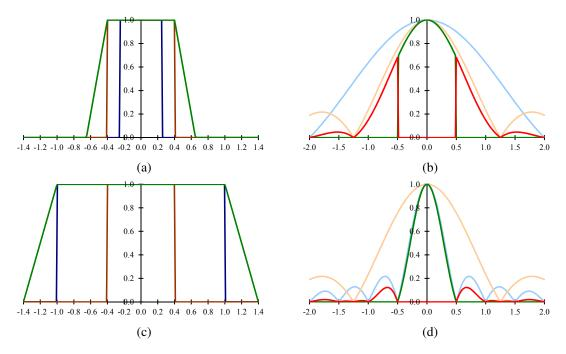
**Figure 2.26** Sample point spread functions (PSF): The diameter of the blur disc (blue) in (a) is equal to half the pixel spacing, while the diameter in (c) is twice the pixel spacing. The horizontal fill factor of the sensing chip is 80% and is shown in brown. The convolution of these two kernels gives the point spread function, shown in green. The Fourier response of the PSF (the MTF) is plotted in (b) and (d). The area above the Nyquist frequency where aliasing occurs is shown in red.
