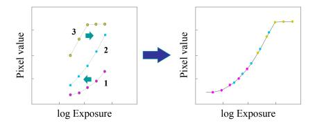
**Figure 10.13** Radiometric calibration using multiple exposures (Debevec and Malik 1997). Corresponding pixel values are plotted as functions of log exposures (irradiance). The curves on the left are shifted to account for each pixel's unknown radiance until they all line up into a single smooth curve.
