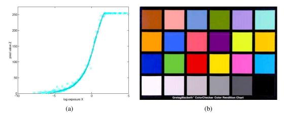
**Figure 10.3** Radiometric response calibration: (a) typical camera response function, showing the mapping between incoming log irradiance (exposure) and output eight-bit pixel values, for one color channel (Debevec and Malik 1997) © 1997 ACM; (b) color checker chart.
