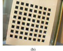
**Figure 6.8** Calibration patterns: (a) a three-dimensional target (Quan and Lan 1999) © 1999 IEEE; (b) a two-dimensional target (Zhang 2000) © 2000 IEEE. Note that radial distortion needs to be removed from such images before the feature points can be used for calibration.
