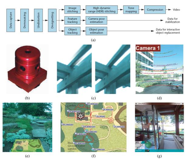
**Figure 13.16** Video-based walkthroughs (Uyttendaele, Criminisi, Kang *et al.* 2004) © 2004 IEEE: (a) system diagram of video pre-processing; (b) the Point Grey Ladybug camera; (c) ghost removal using multi-perspective plane sweep; (d) point tracking, used both for calibration and stabilization; (e) interactive garden walkthrough with map below; (f) overhead map authoring and sound placement; (g) interactive home walkthrough with navigation bar (top) and icons of interest (bottom).
