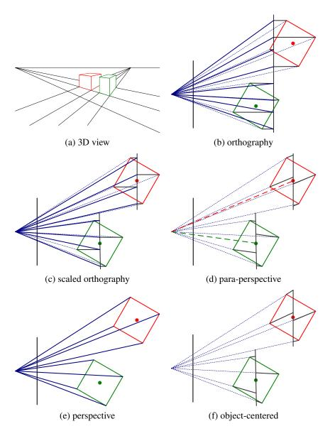
**Figure 2.7** Commonly used projection models: (a) 3D view of world, (b) orthography, (c) scaled orthography, (d) para-perspective, (e) perspective, (f) object-centered. Each diagram shows a top-down view of the projection. Note how parallel lines on the ground plane and box sides remain parallel in the non-perspective projections.
