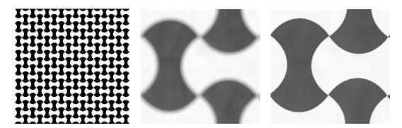
**Figure 10.7** Calibration pattern with edges equally distributed at all orientations that can be used for PSF and radial distortion estimation (Joshi, Szeliski, and Kriegman 2008) © 2008 IEEE. A portion of an actual sensed image is shown in the middle and a close-up of the ideal pattern is on the right.
