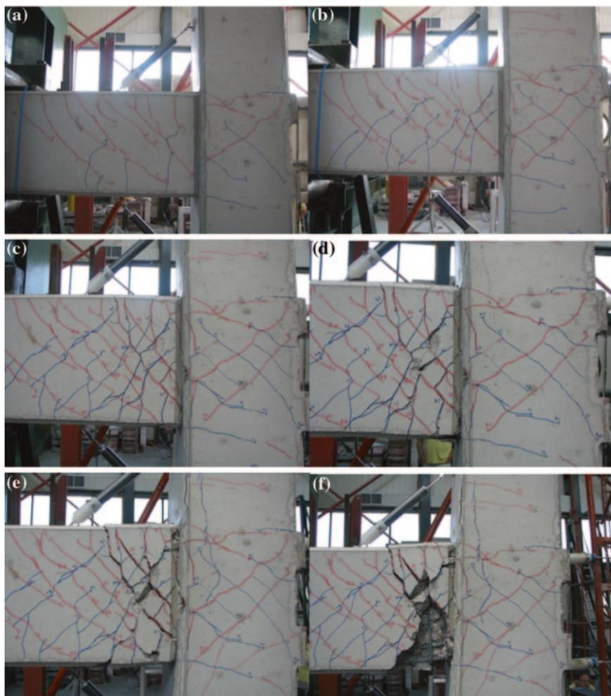
**Fig. 7.21** Crack pattern of specimen S6 at the end of the cyclic stages at maximum displacements equal to (a) 25 mm, (b) 50 mm, (c) 75 mm, (d) 100 mm, (e) 125 mm, and (f) 150 mm
