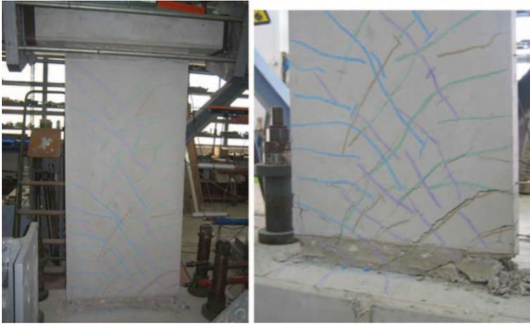
**Fig. 7.15** Typical failure mode of walls under cyclic loading with the location of failure indicated in a magnified form at the *bottom*
