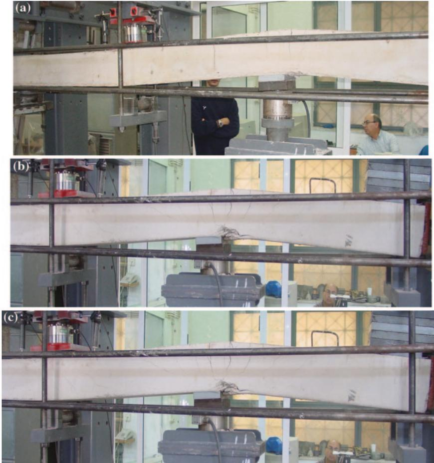
**Fig. 7.28** Modes of failure and associated crack patterns for D14 specimens tested under monotonic loading: **a** ACI-D14-M; **b** EC-D14-M; **c** CFP-D14-M
