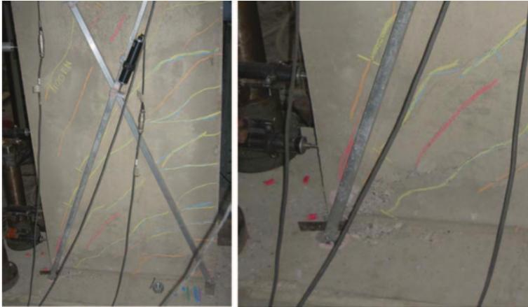
Fig. 7.14 Typical failure mode of walls under monotonic loading with the location of failure indicated in a magnified form at the *bottom*
