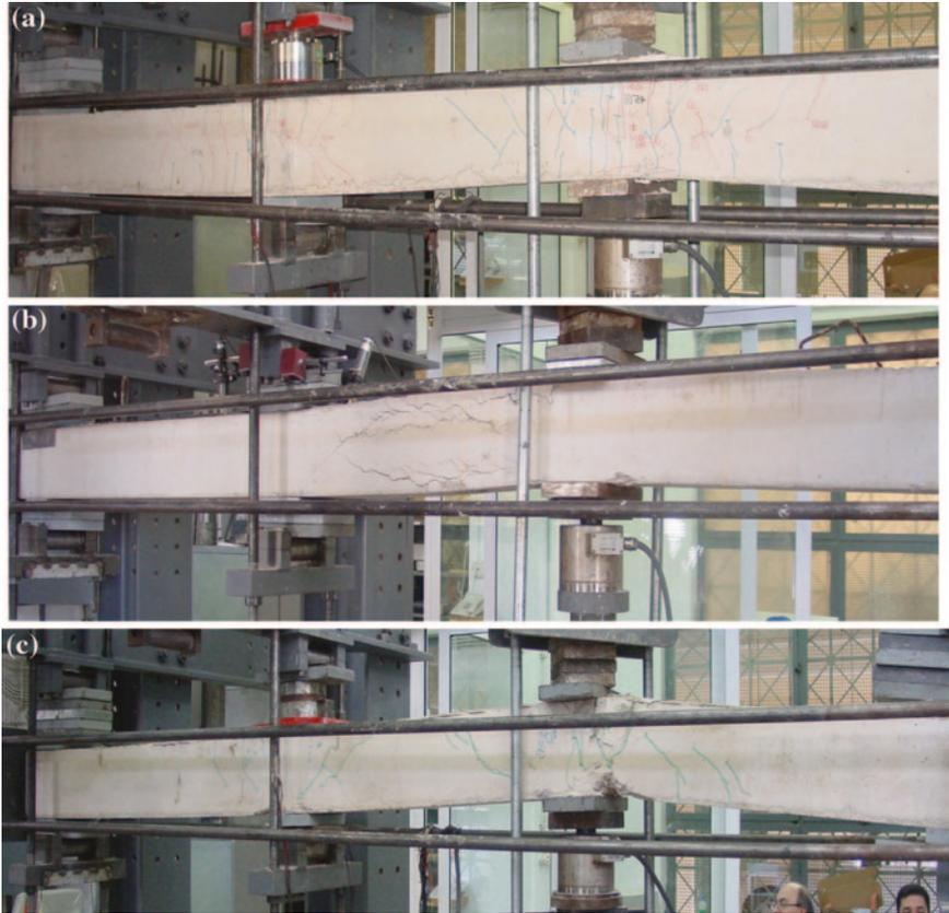
**Fig. 7.30** Modes of failure and associated crack patterns for D14 specimens tested under cyclic loading: **a** Specimen ACI-D14-C; **b** specimen EC-D14-C; **c** specimen CFP-D14-C
