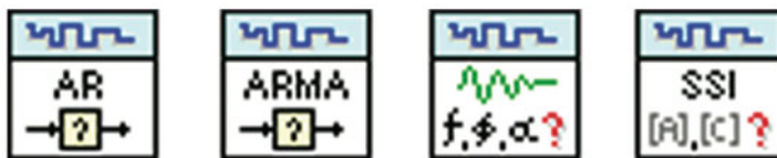
Fig. 1.4 VIs for output-only modal identification (included in the Time Series Analysis Tools)
