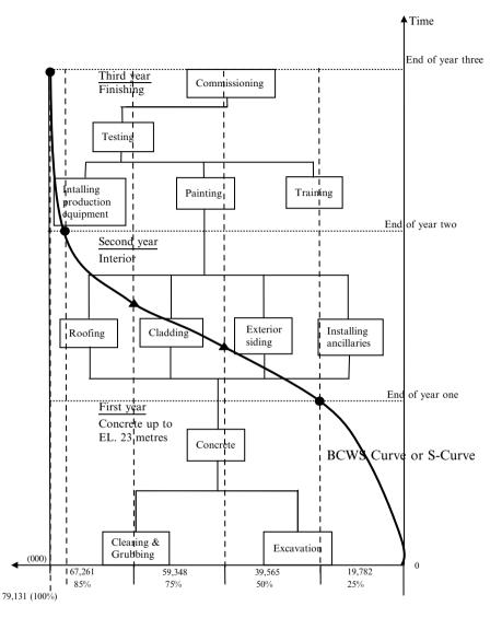
Fig. 5.12 Partial work breakdown structure for the brewery with budget cost of work schedule (BCWS) curve
