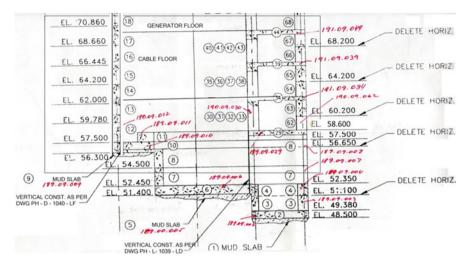
Fig. 8.1 Actual concrete work done for hydroelectric turbine installation
