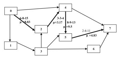
Fig. 3.2 Network using probabilistic values for durations
