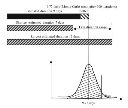
Fig. 2.4 Task duration range and mean for 95 % of confidence level
