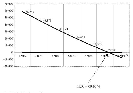
Fig. 5.1 NPV for different discount rates
