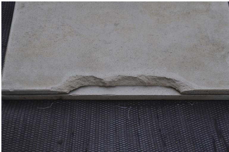
**Fig. 8.7** Slab's edge after tested with a strap anchor
