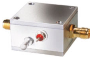
Fig. 5.21. A RF amplifier to be matched to a 50\ \Omega at both the input and output.
