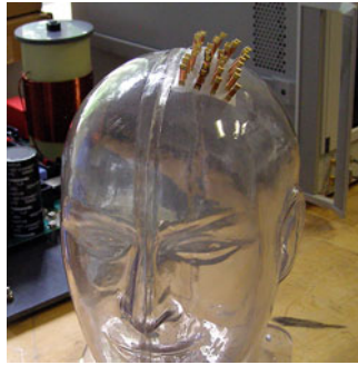
Fig. 12.21. An array of coupled inductors (small coils) located on top of a human-head phantom. This hypothetical setup was tested for applications related to brain stimulation.
