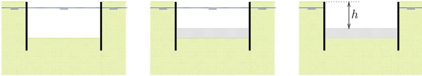
Fig. 9.2 Excavation with concrete floor under water
