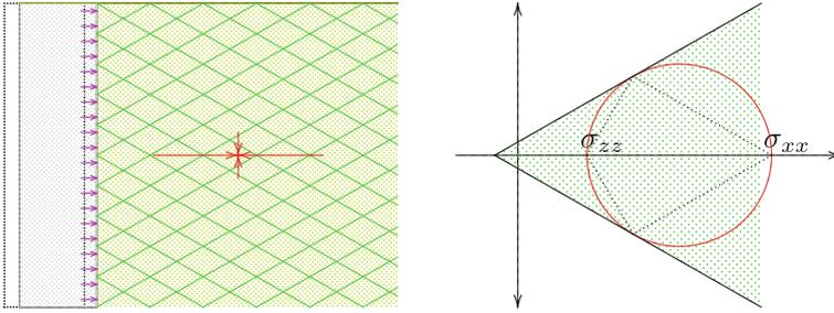
**Fig. 32.6** Passive earth pressure
