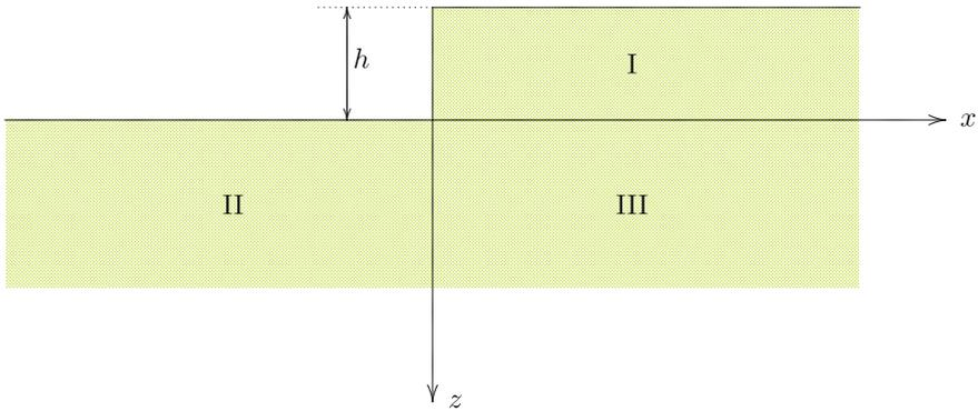
Fig. 43.1 Vertical slope
