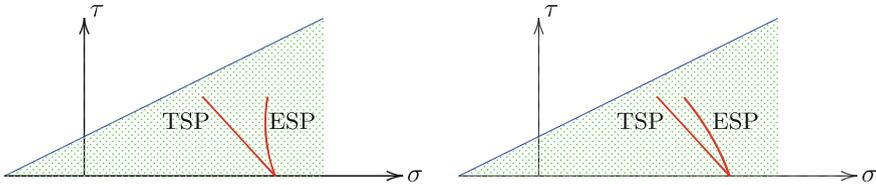
Fig. 25.7 Stress paths in extension tests on dilatant and contractant material
