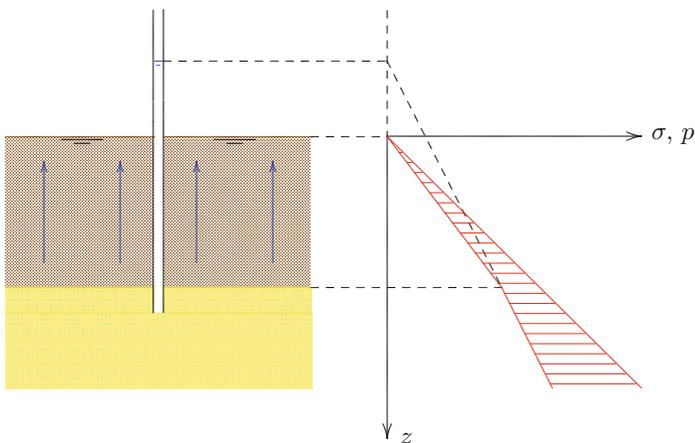
Fig. 8.2 Upward flow, Example 1
