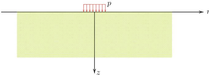
Fig. 27.3 Uniform load over circular area
