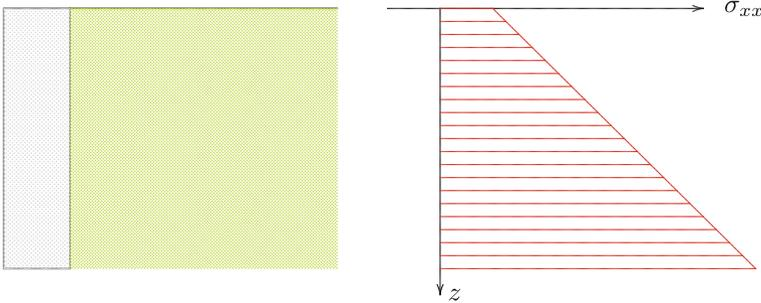
**Fig. 32.7** Horizontal stresses in case of passive earth pressure
