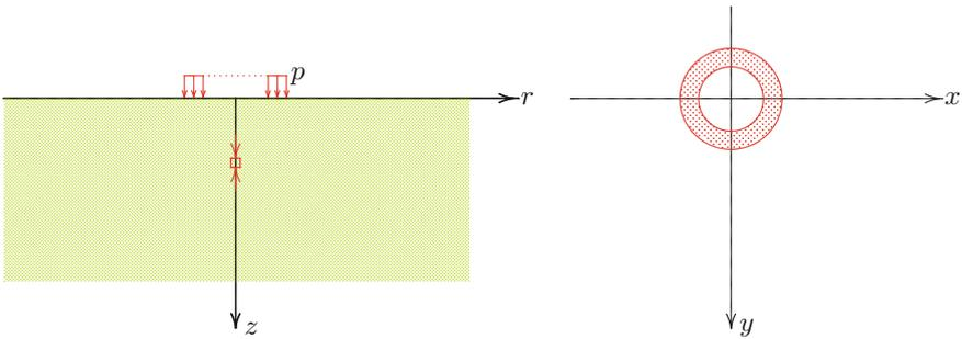
**Fig. 28.2** Uniform load on a ring
