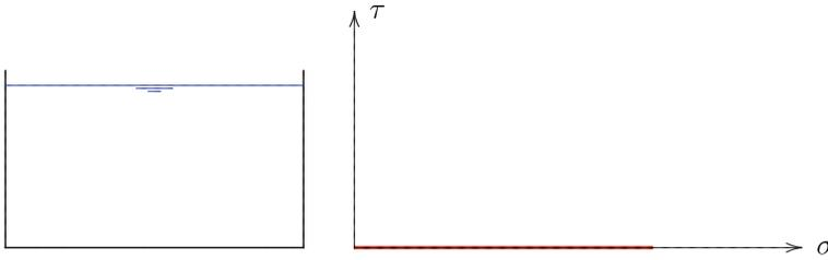
**Fig. 31.2** Stress path for a fluid
