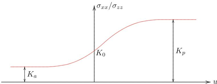
Fig. 32.9 Horizontal stress as a function of the displacement
