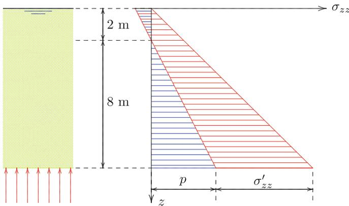
Fig. 5.4 Lowering the phreatic surface by 2 m, with capillary rise
