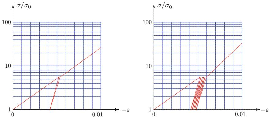
**Fig. 14.3** Loading, unloading, and cyclic loading
