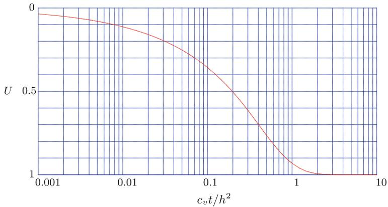
**Fig. 16.3** Degree of consolidation
