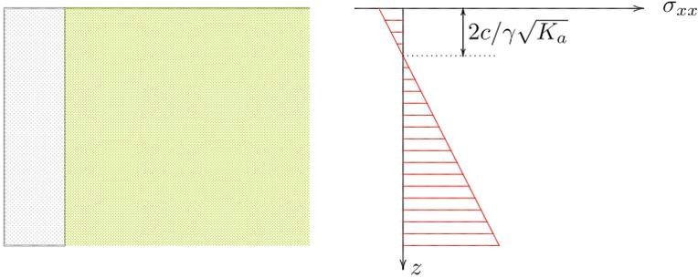
**Fig. 32.4** Horizontal stress in case of active earth pressure
