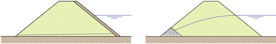
**Fig. 44.7** Dam with a clay blanket, or with a drain
