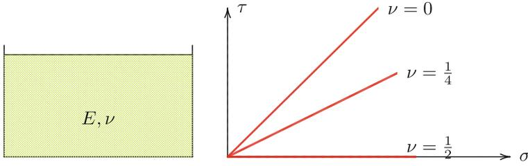
**Fig. 31.3** Stress path for elastic material
