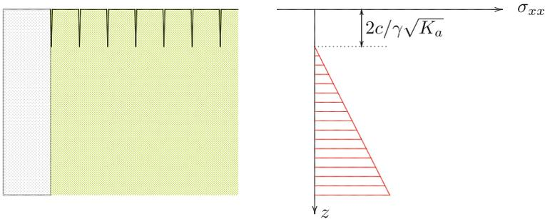
**Fig. 32.5** Horizontal stresses, with cracks in the soil
