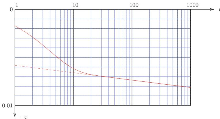
**Fig. 19.1** Primary and secondary consolidation
