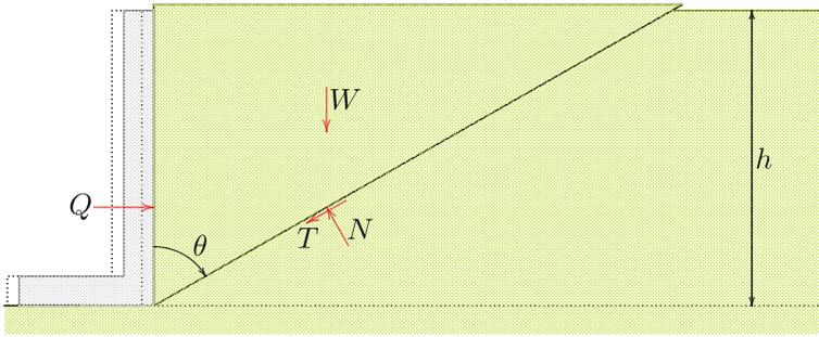
Fig. 33.2 Passive earth pressure
