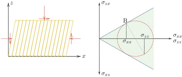
Fig. 41.3 Shearing on vertical planes: the book row mechanism
