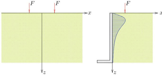
**Fig. 29.4** Line load next to a smooth rigid wall
