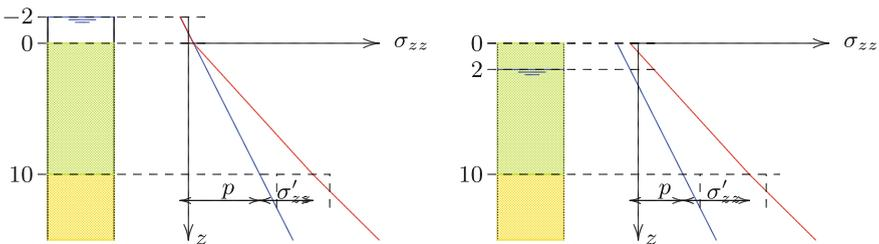
**Fig. 5.7** Stresses before and after lowering the water table
