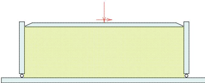
Fig. 22.4 Simple shear test
