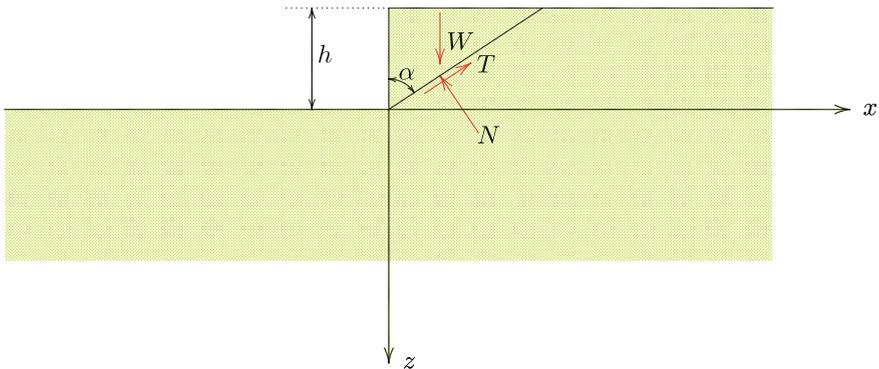
Fig. 43.3 Mechanism with straight slip surface
