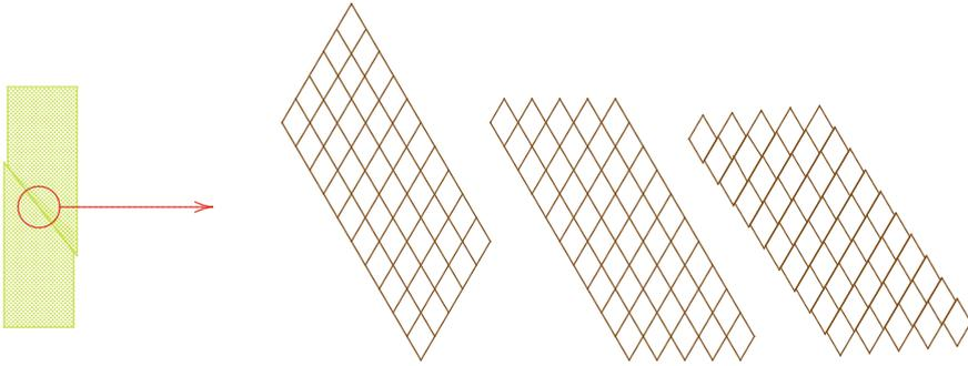
**Fig. 21.6** Apparent shear plane in triaxial test
