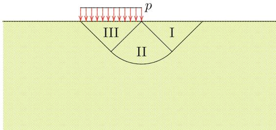
Fig. 40.2 Prandtl's schematization
