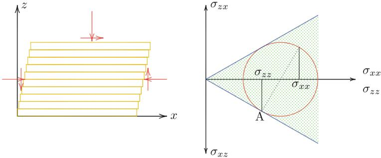
Fig. 41.2 Shearing on horizontal planes
