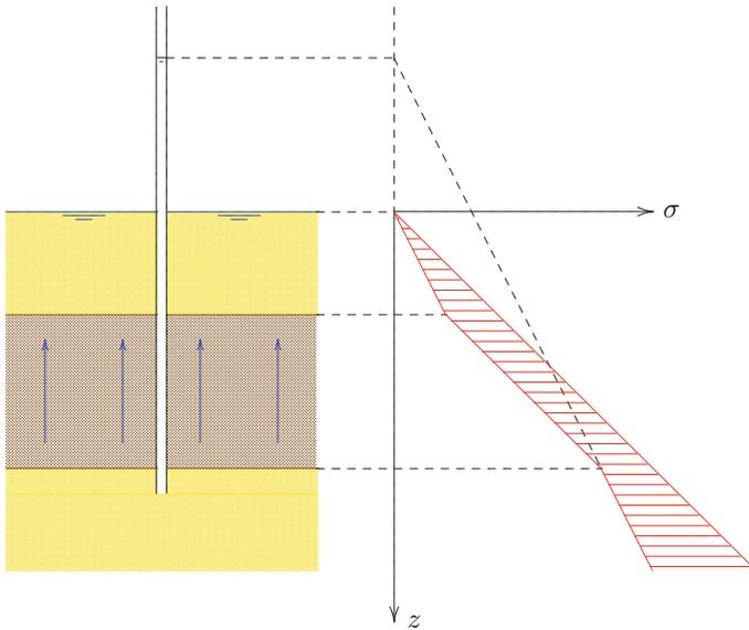
Fig. 8.4 Upward flow, Example 2
