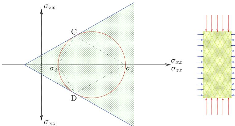
Fig. 21.4 Mohr's circle for the triaxial test
