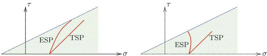
**Fig. 25.4** Stress paths in triaxial tests on dilatant and contractant material
