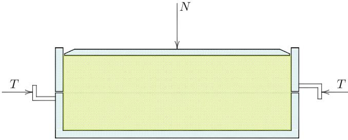
Fig. 22.1 Direct shear test
