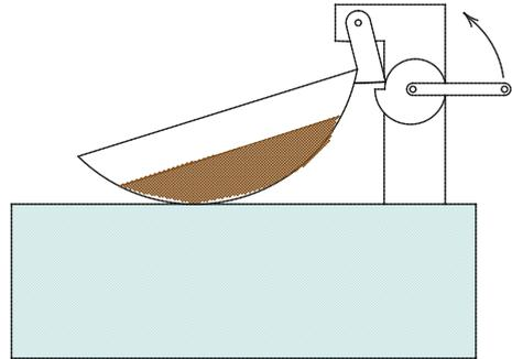
perhaps mixing the clay some more, the water content will have decreased, and the test may be repeated, until the groove is closed after precisely 25 drops. Then the water content must immediately be determined, before any more water evaporates, of course.
