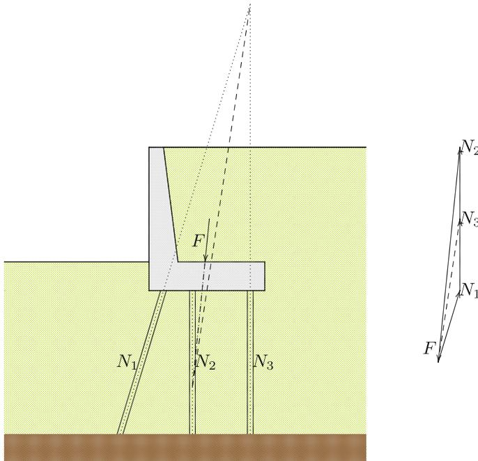
Fig. 48.2 Statically determinate pile foundation
