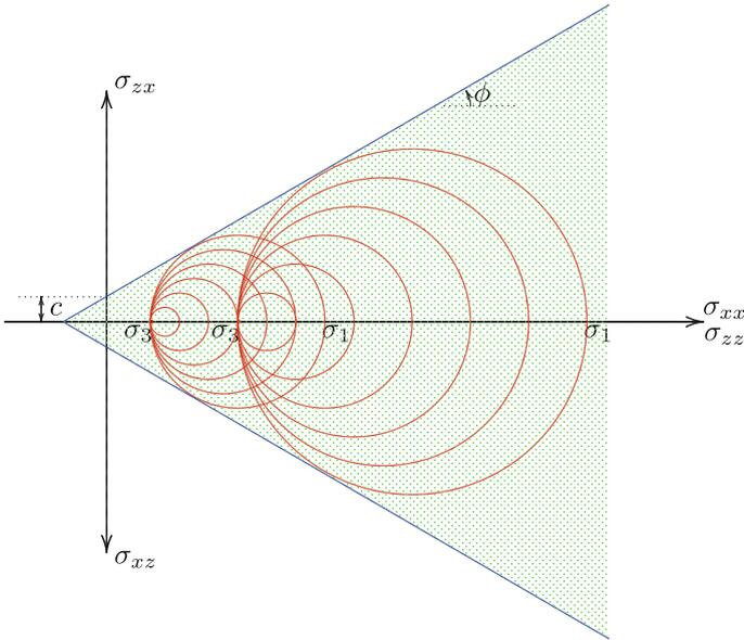
Fig. 21.5 Determination of  $c$  and  $\phi$  from two tests
