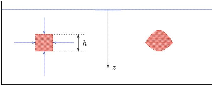
**Fig. 9.1** Archimedes' principle
