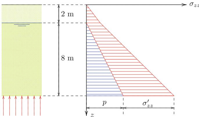
Fig. 5.5 Lowering of the phreatic surface by 2 m, no capillarity
