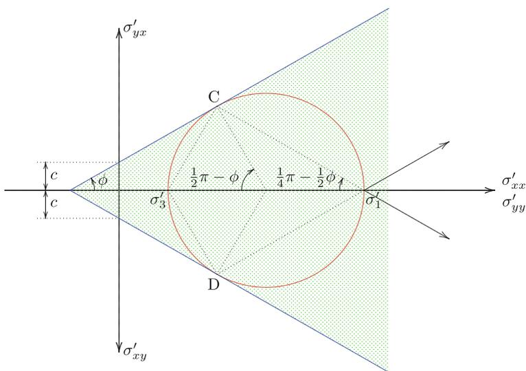
Fig. 20.4 Mohr–Coulomb failure criterion
