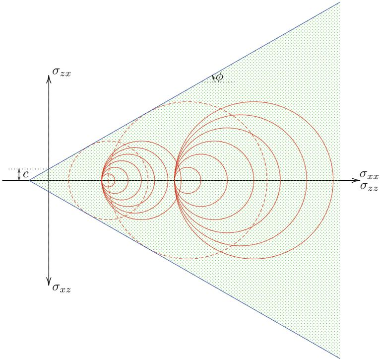
**Fig. 23.2** Determination of  $c$  and  $\phi$  from two tests
