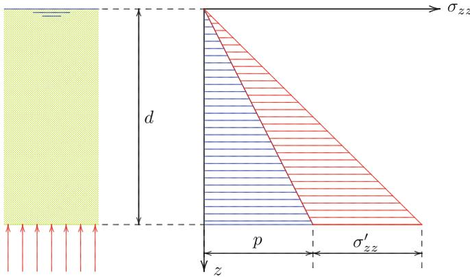
**Fig. 5.1** Stresses in a homogeneous layer
