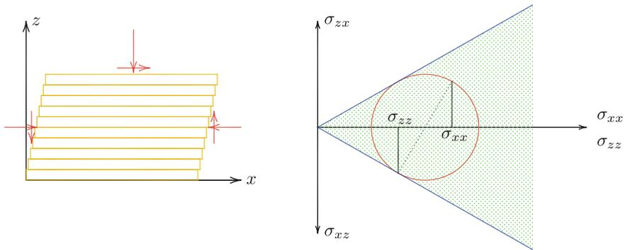
Fig. 22.3 Sliding on horizontal planes
