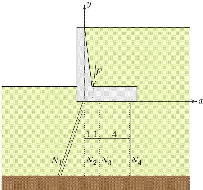
**Fig. 48.3** Statically indeterminate pile foundation
