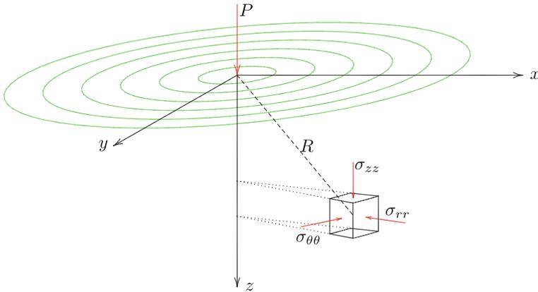
**Fig. 27.1** Point load on half space
