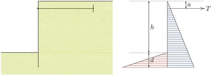
**Fig. 35.1** Anchored sheet pile wall
