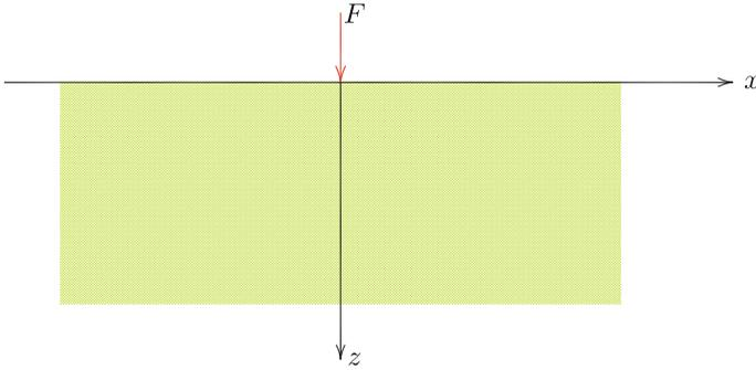
**Fig. B.6** Line load on half space
