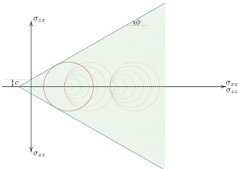
Fig. 24.1 Mohr circles for two undrained tests
