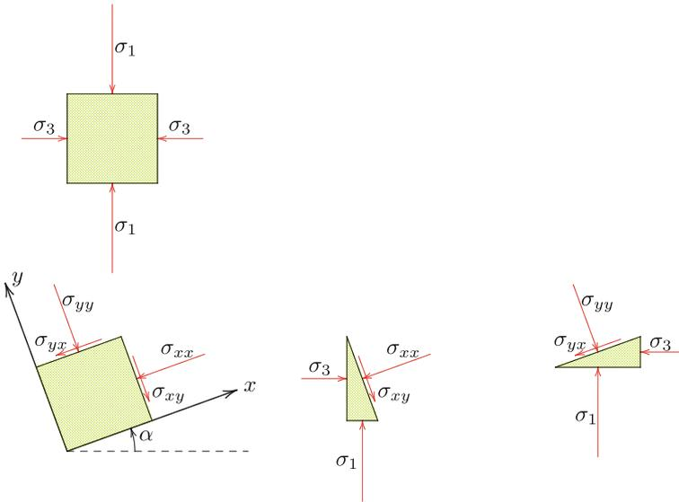
Fig. 20.2 Stresses on a rotated plane
