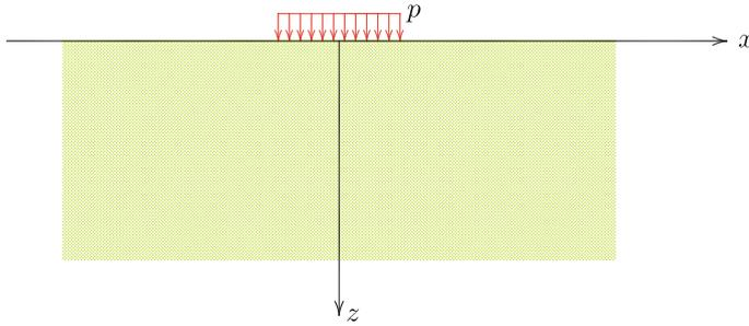
Fig. 39.1 Strip load on half space
