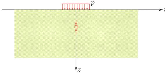
**Fig. 28.1** Uniform load on circular area
