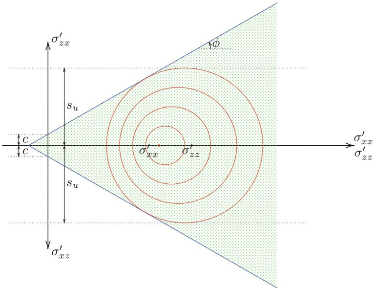
**Fig. 24.6** Mohr circles for undrained behavior
