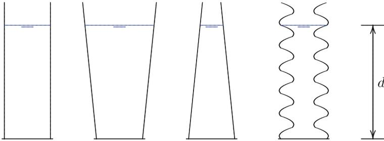
Fig. 4.3 Stevin: hydrostatic water pressure depends upon depth only
