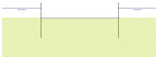
**Problem 10.2** A building pit in a lake is being constructed, using a sheet pile wall surrounding the building pit. Inside the wall the water level is lowered (by pumping) to the level of the ground surface. Outside the sheet pile wall the water level is 5 m higher. It has been installed to a depth of 10 m below ground surface. The thickness of the soil layer is 20 m. Sketch a flow net, and determine the maximum gradient inside the sheet pile wall.
