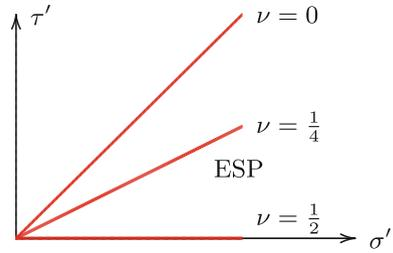
**Fig. 31.6** Elastic material under water
