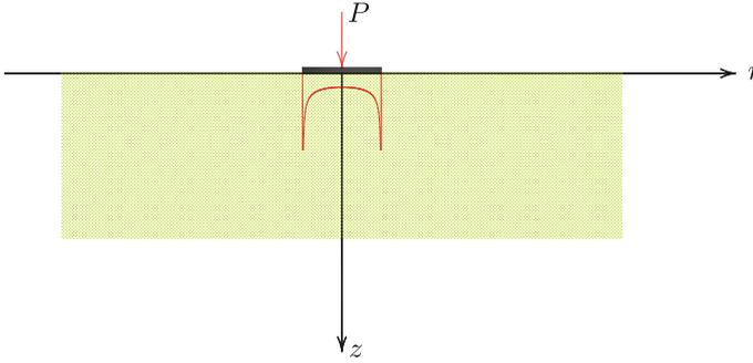
Fig. 27.4 Rigid plate on half space
