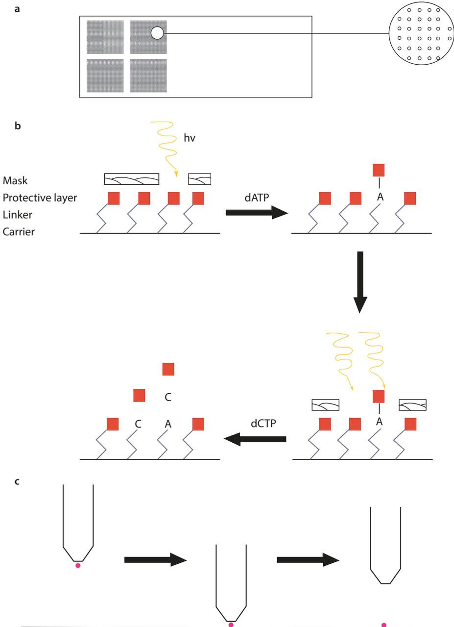
**Fig. 6.2** DNA microarrays. **a** DNA microarray that consists of several thousand nucleic acid spots and arrayed in high density. **b** Schematic illustration of production of an oligonucleotide array using photolithography. **c** cDNA solutions are spotted during array production onto microarray plates by robots
