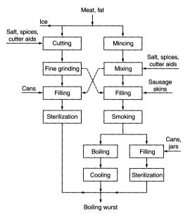
Fig. 12.34. Production of boiling sausage ("Brüh-wurst")
