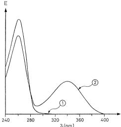
**Fig. 2.5.** Electron excitation spectra of NAD (1) and NADH (2)
