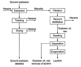
Fig. 14.2. Production of oil and lecithin from soybeans
