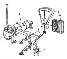
**Fig. 15.25.** Farinograph (according to *Rohrlich* and *Thomas*, 1967). The apparatus consists of a thermostated mixer or kneader (1), its blades are driven by an electromotor (2). The reaction torque acts through a lever system (4) of analytical balance precision on the indicator scale (5) simultaneously recorded on a strip chart recorder (6). The movement of the lever system is damped by an oil dash pot (3). The farinogram is a diagram of force versus time
