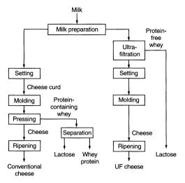
Fig. 10.26. Cheese making (conventional or with ultrafiltration)
