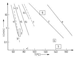
**Fig. 10.15.** Heating of milk. I-3 Pasteurization: I high temperature treatment, 2 short time and 3 long time heat treatment; 4 and 5 UHT treatment: 4 indirect and 5 direct; 6 sterilization. *a*: Killing pathogenic microorganisms (*Tubercle bacilli* as labelling organism), *b/c*: inactivation of alkaline/acid phosphatase.  $d_1$ ,  $d_2$ ,  $d_3$  denaturation (5, 40, 100%) of whey proteins. *e*: casein heat coagulation, *f*: start of milk browning
