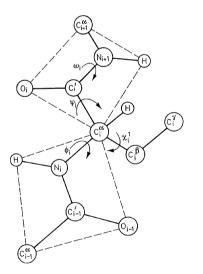
Fig. 1.16. Definitions for torsion angles in a peptide chain
