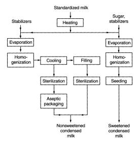
Fig. 10.25. Production of condensed milk
