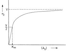
**Fig. 2.22.** Determination of *Michaelis* constant, K<sub>m</sub>, according to Equation (2.41)
