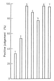
**Fig. 4.7.** Sensory evaluation of canned cherries prepared with different sweeteners 1, 2, 3: 60, 50, 40% saccharose, 4: 0.15% cyclamate, 5: 0.05% saccharin, 6: 10% saccharose + 0.10% cyclamate, 7: 10% saccharose + 0.02% saccharin (according to *Salunkhe*, 1963)
