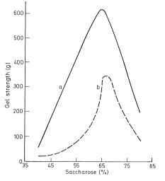
**Fig. 4.24.** Gel strength of (*a*) tamarind flour and (*b*) pectin from lemons versus saccharose concentration (according to *Whistler*, 1973)
