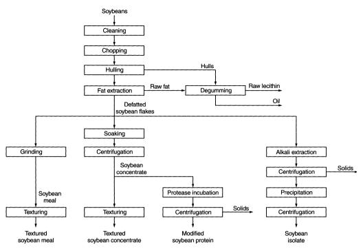
Fig. 16.6. Soybean processing
