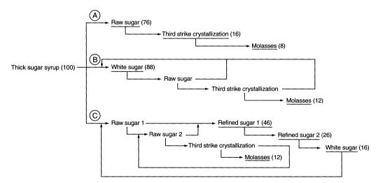
**Fig. 19.7.** Crystallization scheme for the production of A) raw sugar, B) white sugar, and C) refined sugar. The yields of sucrose (%), based on the amount of sucrose added with the thick syrup, are given in brackets behind the final products (*underlined*)
