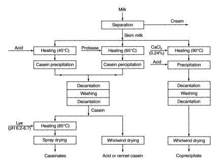
Fig. 10.30. Production of casein, caseinates, and coprecipitate
