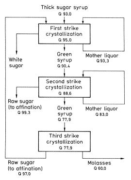
**Fig. 19.8.** White sugar evaporation and crystallization. Quotient Q: % saccharose in dry matter
