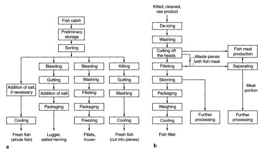
Fig. 13.4. Fish processing on board (a) and on land (b)
