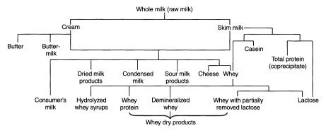
Fig. 10.19. Schematic presentation of milk processing
