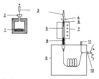
**Fig. 5.9.** Apparatus for the gas chromatography–olfactometry of static headspace samples. *1* Sample in thermostated glass vessel, 2 septum, 3 gastight syringe, 4 injector, 5 hydrophobed glass tube, 6 carrier gas, e.g., he-lium, 7 purge and trap system, 8 cold trap, 9 gas chromatograph with capillary column, *10* sniffing port, *11* flame ionization detector (according to *Guth* and *Grosch*, 1993)
