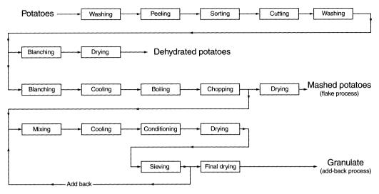
Fig. 17.4. Production of dehydrated potatoes, mashed potato flakes and potato granulate
