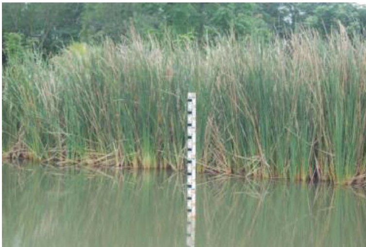
Forebay depth measurement is required annually
