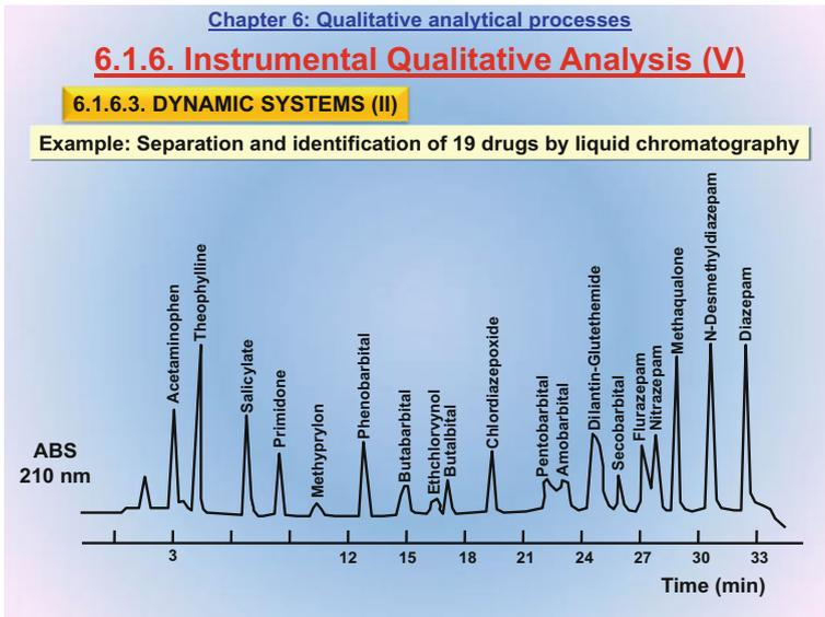
This slide illustrates the potential of liquid chromatography for multi-identification with the separation and identification of 19 drugs in human serum. Although some peaks in the chromatogram are overlapped, their retention times are different enough for qualitative identification purposes.
