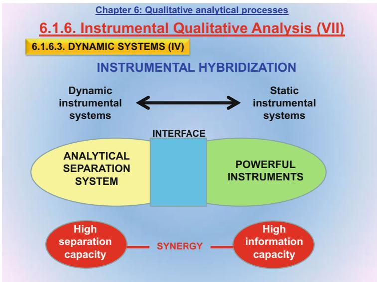
So-called *instrumental hybridization* is the synergistic combination of two or more instrument systems in order to boost their individual qualitative and quantitative information potentials. The key to an effective connection here is finding an appropriate interface with a view to maximizing analyte separation and information production.
