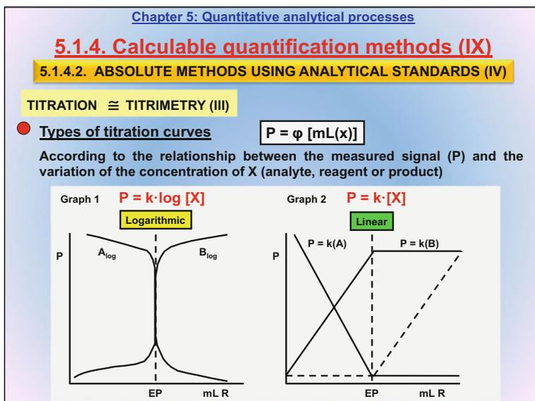
A *titration curve* is constructed by plotting the analytical signal against the volume of titrant added. The signal can vary in a logarithmic (graph 1) or linear manner (graph 2) with the analyte concentration depending on whether the relationship between the instrument response and the concentration of the monitored species is of the proportional or logarithmic type.
