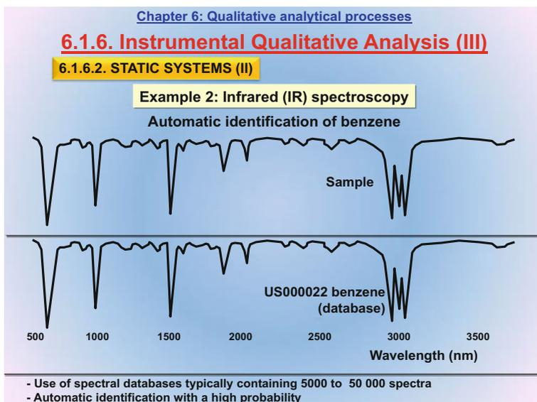
This slide illustrates the automatic identification of benzene by infrared (IR) absorption spectroscopy, which is a widely used technique for qualitative analytical purposes.
