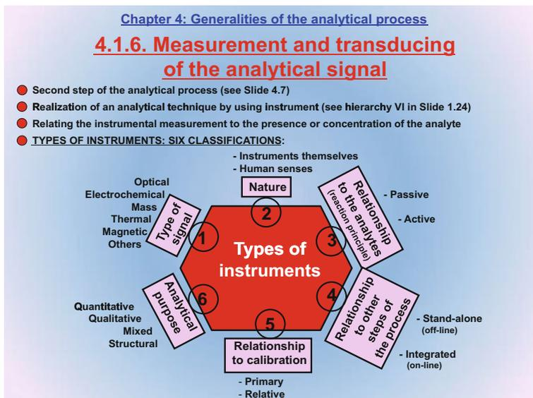
The second step of the analytical process (see Slide 4.7) involves measuring and transducing<sup>1</sup> the analytical signal (primary data), which is processed to obtain the analytical results in the third. This operation requires using a measuring instrument (see the hierarchy in Slide 1.24).
