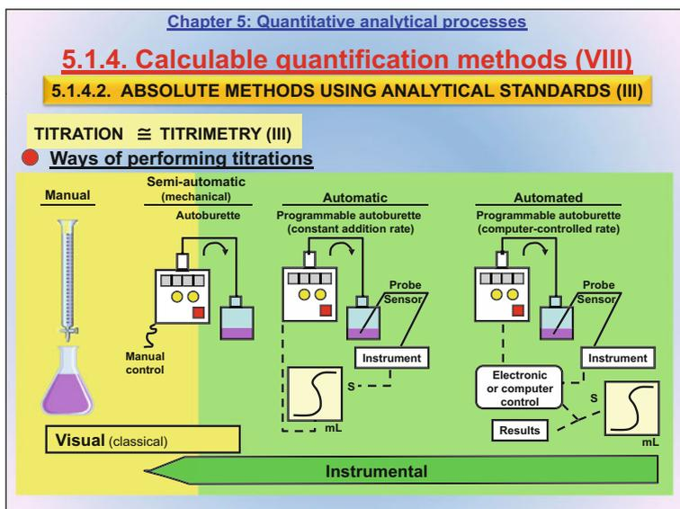
Automation has also reached titrations and titrimetries. In the process, formerly manual work has been rendered automatic. This slide compares three different types of autoburettes with a classical burette.
